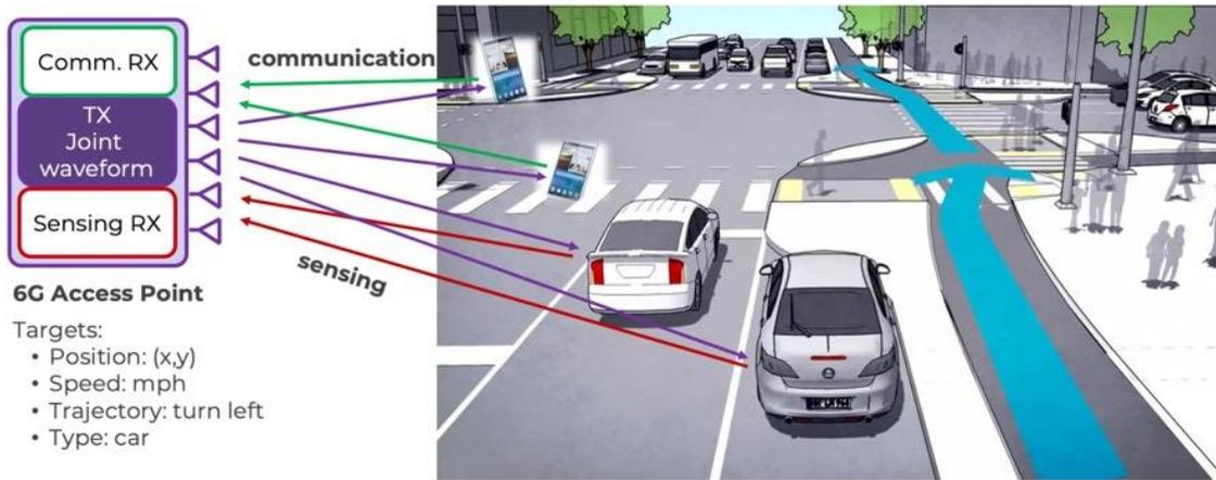
Figure 2: Joint sensing and communication in a vehicular scenario (monostatic configuration).
