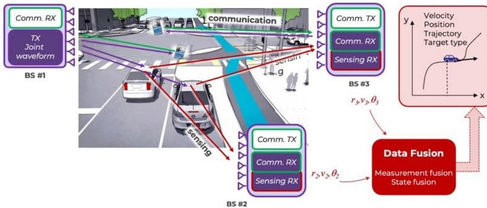
Figure 3: Joint sensing and communication in a vehicular scenario (multi-static/distributed configuration).
