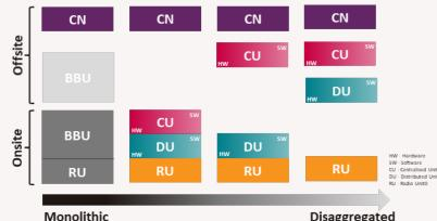
Disaggregation includes decoupling of HW/SW in addition to disaggregating network elements Open RAN connects disaggregated RAN elements through the use of open & interoperable interfaces
