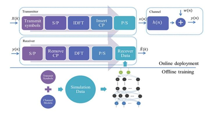
Input: received pilot OFDM block + received data OFDM block
