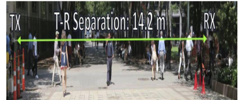
Pedestrian blockage at 73GHz
