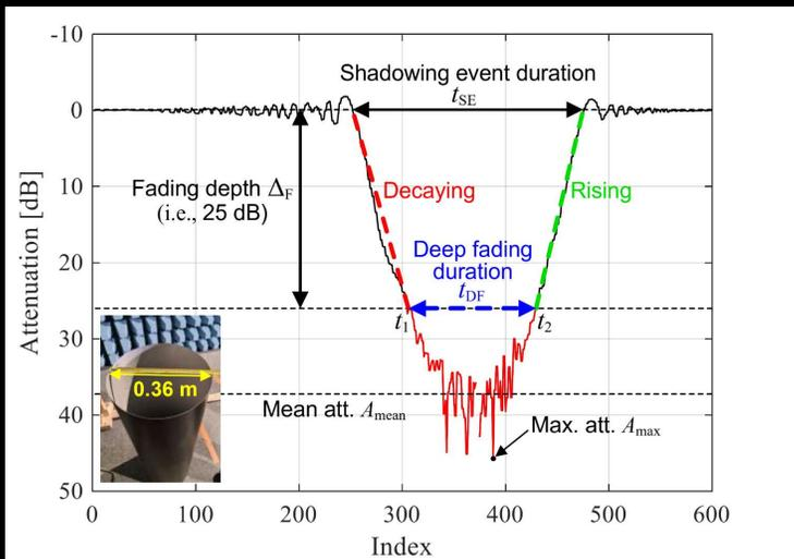
Reference measurement with metallic cylinder
