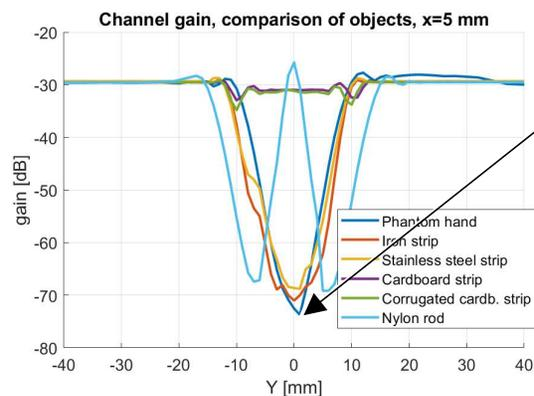
Up to 44.2 dB attenuation if obstacle is 5 mm from antennas
