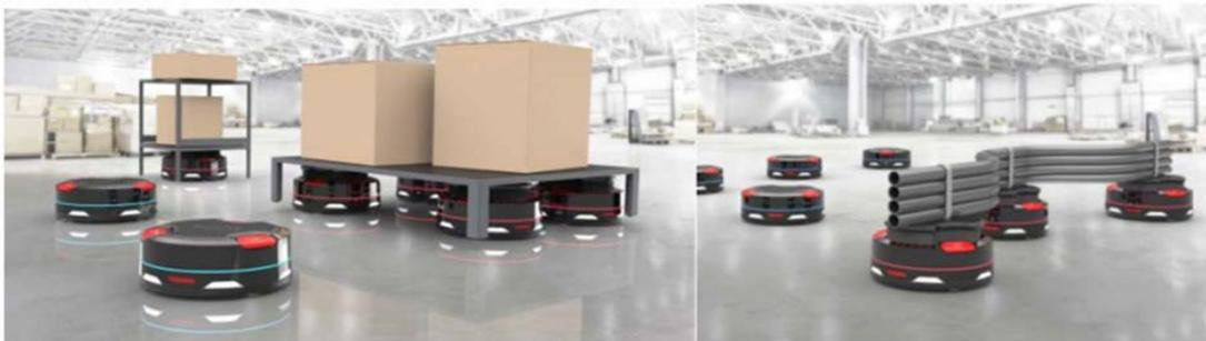
Figure 12: Illustration of the AMR testbed for handling pallets with varying sizes and shapes.
