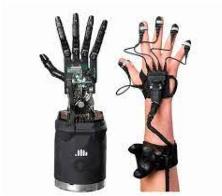
Figure 14: Dexterous Robotic Hands & Operator Terminal Equipment [Shadow Robot]
