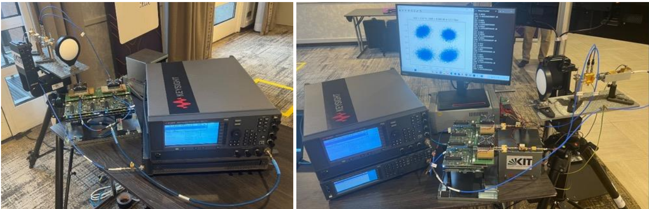
Figure 12: Sub-THz transmission setup: transmitter (left) and receiver (right).
