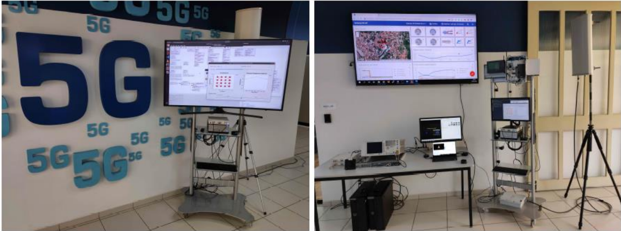
Figure 4: Base station and user terminal used in the 6G network demonstration.
