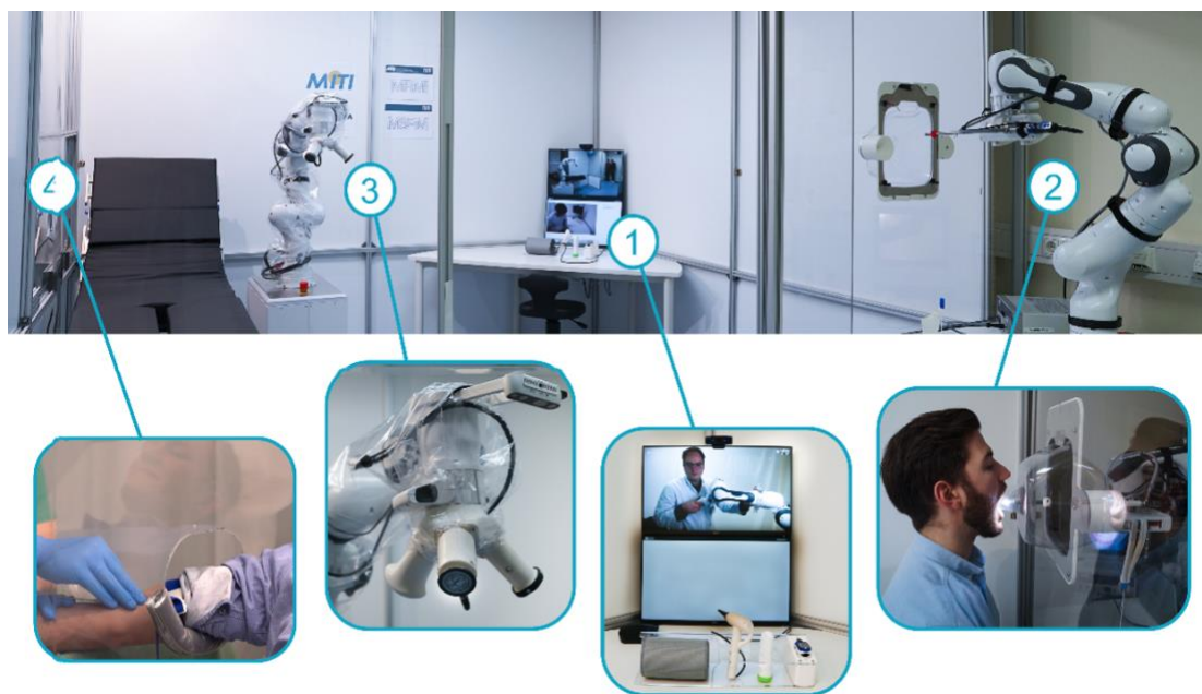
Figure 6: Telerobotic diagnostics framework. (1) Medical history and vital parameter assessment. (2) Robotic oral cavity inspection and swab sampling. (3) Bilateral multifunctional teleoperation system. (4) Safety hatch for additional manual diagnostics, e.g. blood sampling. 9
