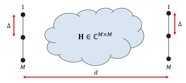
**Problem:** Optimize spacing  $\Delta$  to maximize MIMO capacity High SNR: M equal singular values
