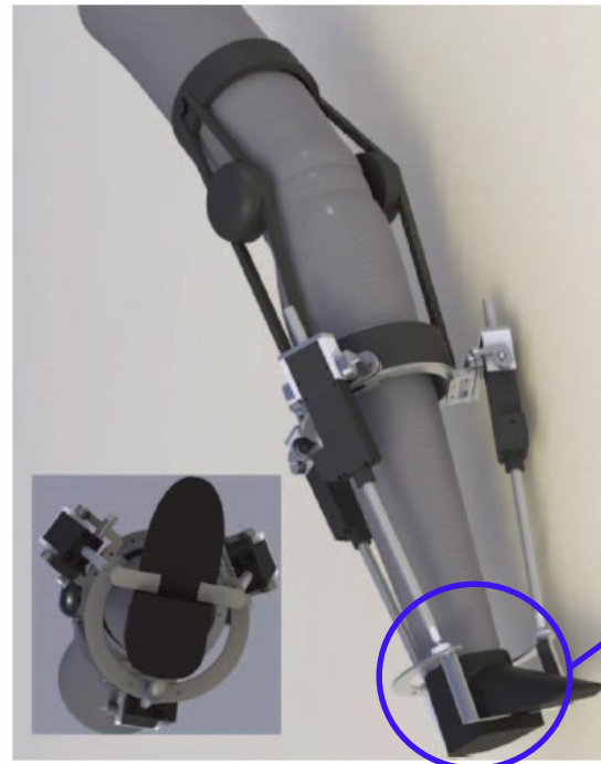
Early prototype of Sukorpion AR robot
