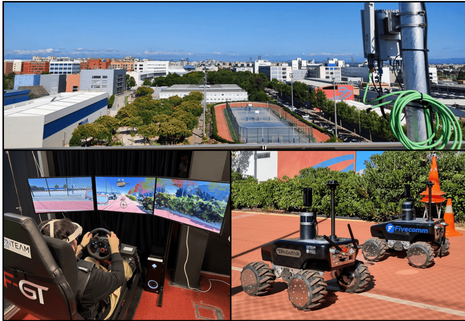
Figure 2: Images illustrating the iTEAM-UPV 6G-enabled DT testbed. (Top): 5G networking infrastructure. (Bottom left): a human operator controlling a mobile robot via an immersive interface with VR, AR and haptic elements. (Bottom right): two Robotnik Summit XL robots, linked via 5G to human operators.
