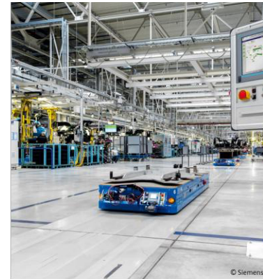
Flexible Modular Assembly Area Communication of mobile assets (AGVs, mobile robots, ...)
